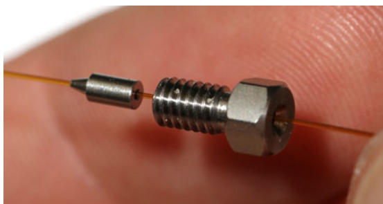
Figure 406. Positioning the Nut and Ferrule Correctly on the Column
