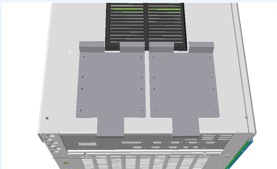
Figure 517. Installation of two Support Bracket
