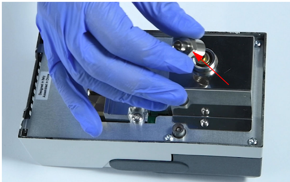
Figure 335. Removing the Injector Bottom Fitting
