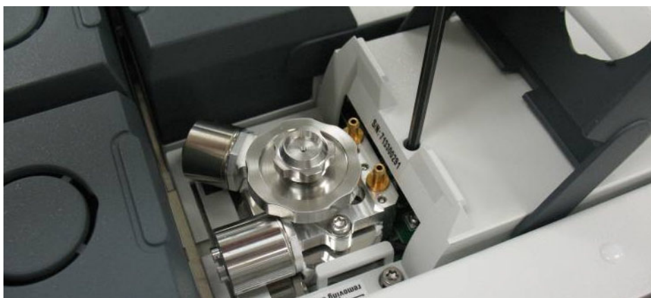
Figure 505. Securing the Instant Connect Helium Saver Injector Module in Place
