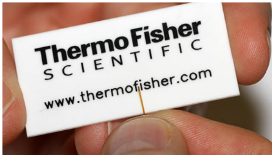
Figure 403. Cutting the Tubing with the Scoring Wafer
