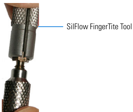
Figure 409. Swaging the Ferrule Using the SilFlow FingerTite Tool
