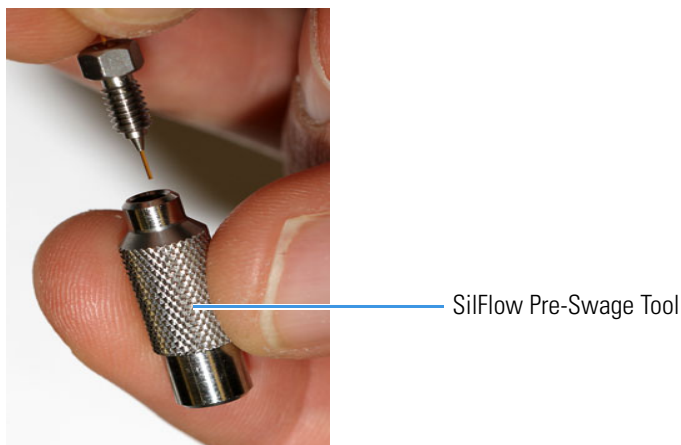
Figure 387. Inserting the Column and Ferrule into the SilFlow Pre-Swage Tool
