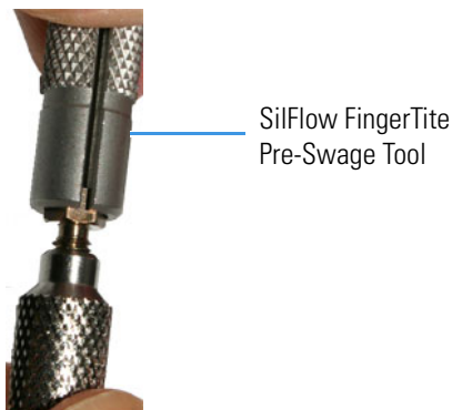
Figure 388. Swaging the Ferrule Using the SilFlow FingerTite Tool
