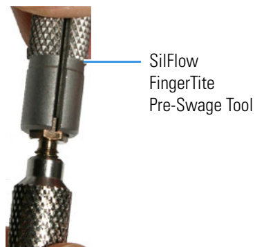
Figure 405. Swaging the Ferrule Using the SilFlow FingerTite Tool
