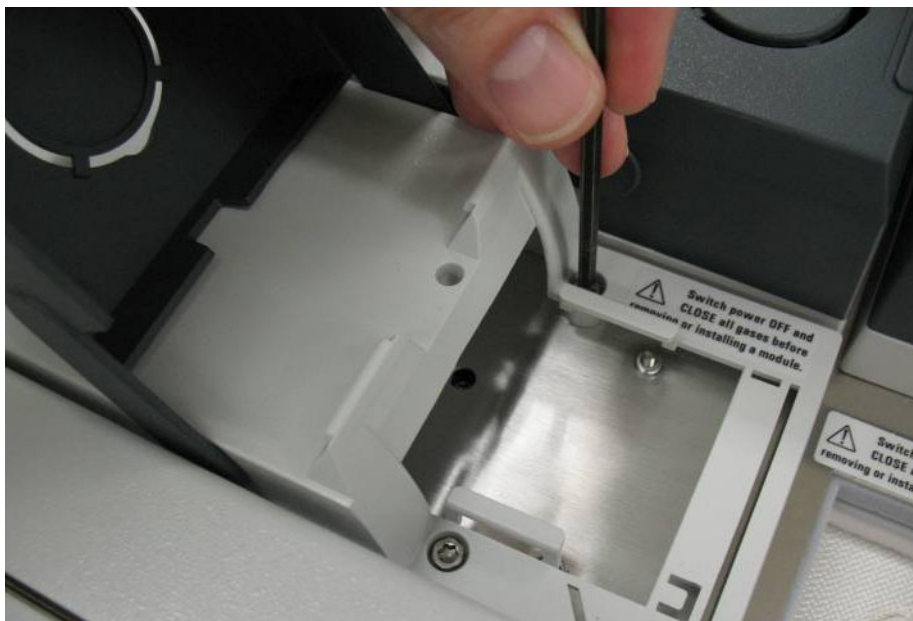
Figure 500. Removing the Dummy Modules
