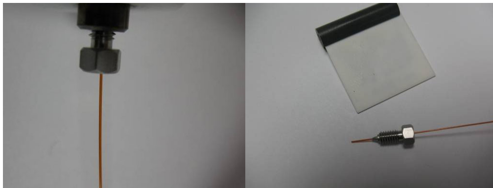
Figure 508. Installing the Column in the Injector
