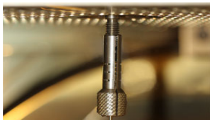
Figure 401. Securing the 30 cm Fused Silica Restrictor to the No-Vent Microfluidics Module
