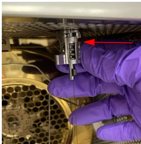
Figure 67. Connecting the iConnect Column Lock to the iConnect Nut
