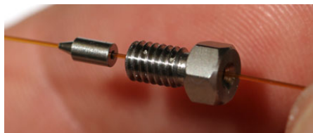
Figure 385. Positioning the SilFlow Nut and SilFlow Ferrule Correctly on the Tubing
