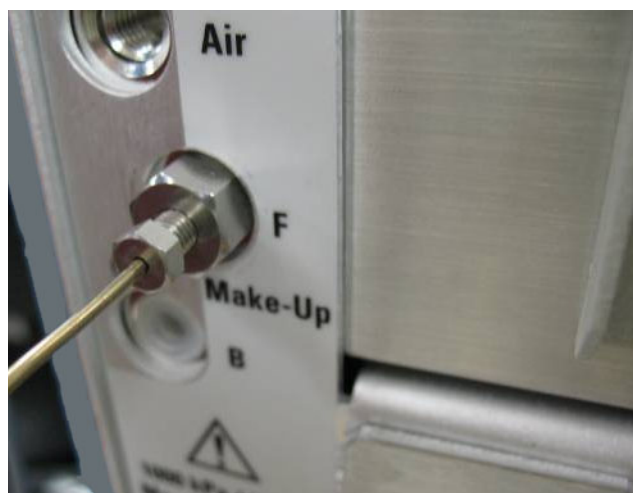
Figure 503. Plumbing the Helium Cylinder
