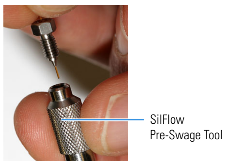
Figure 408. Inserting the Column and Ferrule into the SilFlow Pre-Swage Tool
