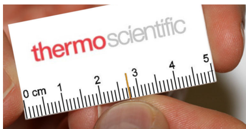
Figure 346. Cutting the Tubing with the Scoring Wafer
