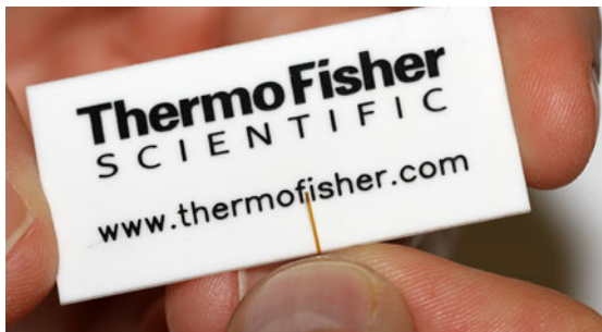
Figure 407. Cutting the Column with the Scoring Wafer
