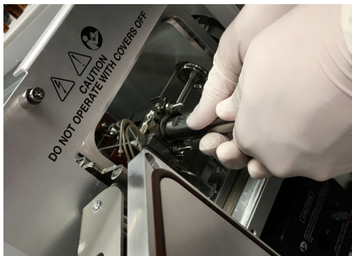
Figure 427. Removing the ExtractaBrite Ion Source
