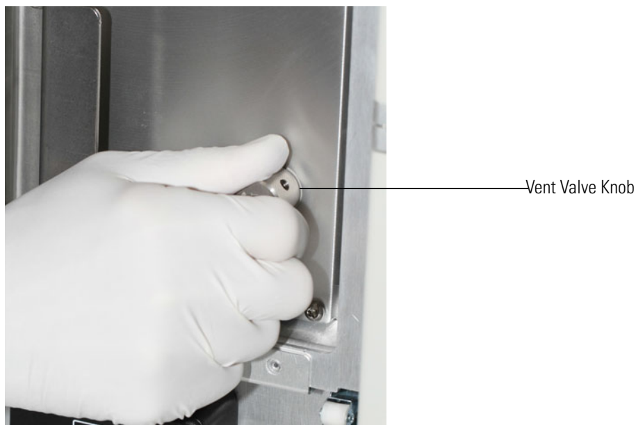
Figure 47. Venting the Mass Spectrometer
