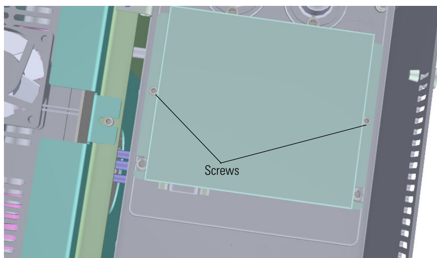
Figure 384. Reattaching the Electrometer Shield
