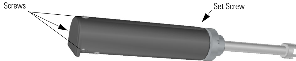
Figure 208. Removing Source Exchange Tool Screws
