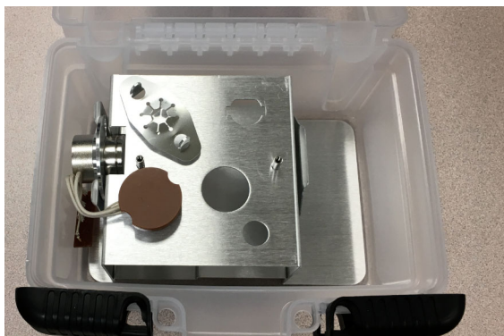
Figure 428. Removing the AEI Source from the Storage
