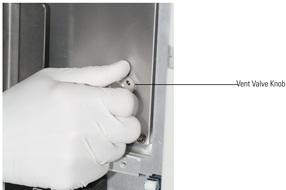
Figure 54. Venting the ISQ 7610 Mass Spectrometer
