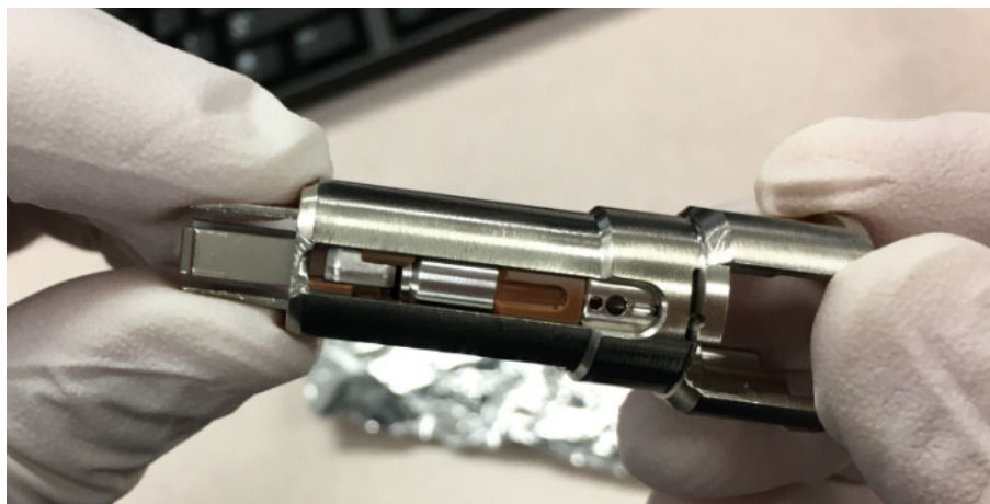
Figure 58. Advanced EI Ion Source Cartridge
