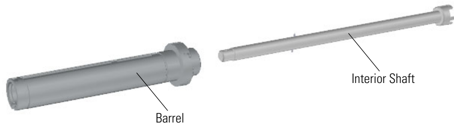
Figure 210. Removing the Interior Shaft
