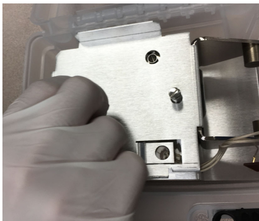
Figure 431. Storing Extra Source Parts in the AEI Source Case
