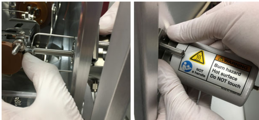
Figure 122. Separating the Transfer Line From the Source Heater Block
