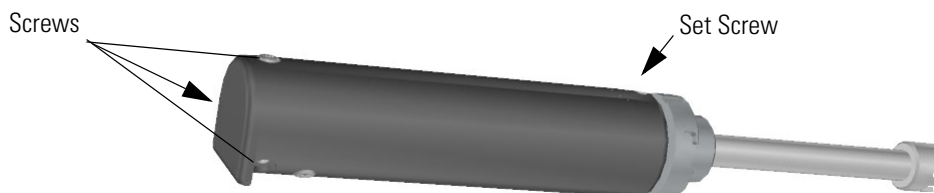
Figure 215. Reattaching the Source Exchange Tool Screws
