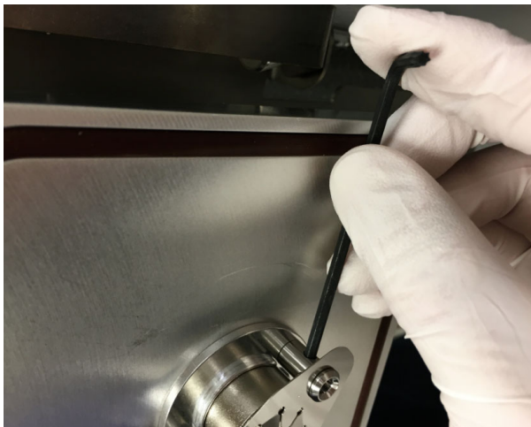
Figure 426. Tightening the Magnets
