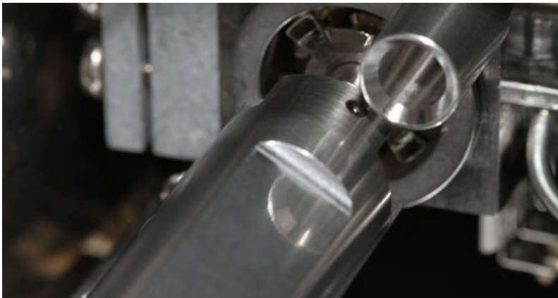
Figure 76. Removing the Small Source Tool from the Instrument
