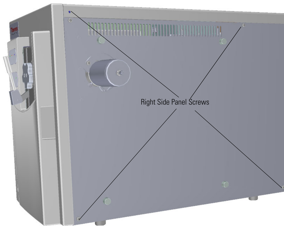
Figure 412. Removing the Right Side Panel Screws
