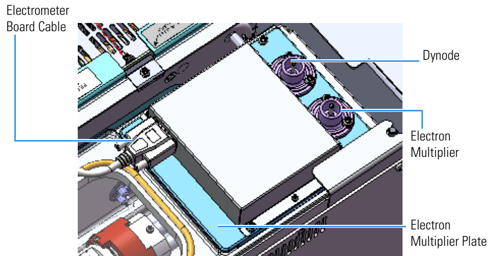
Figure 396. Disconnecting the Electron Multiplier Cables
