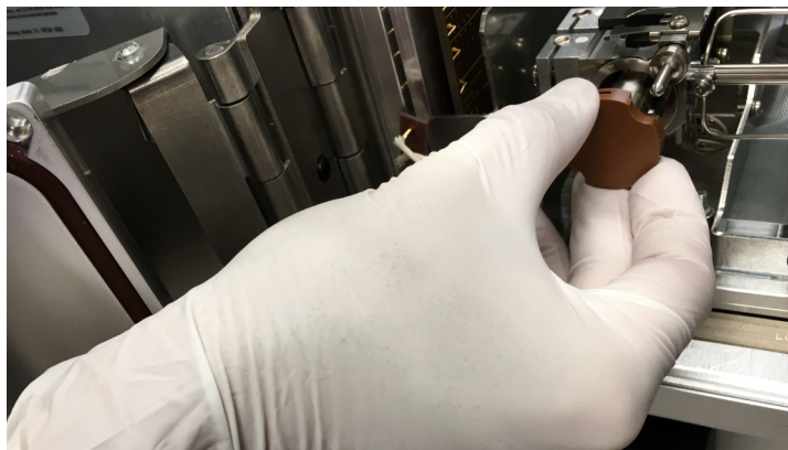
Figure 480. Installing the AEI Source
