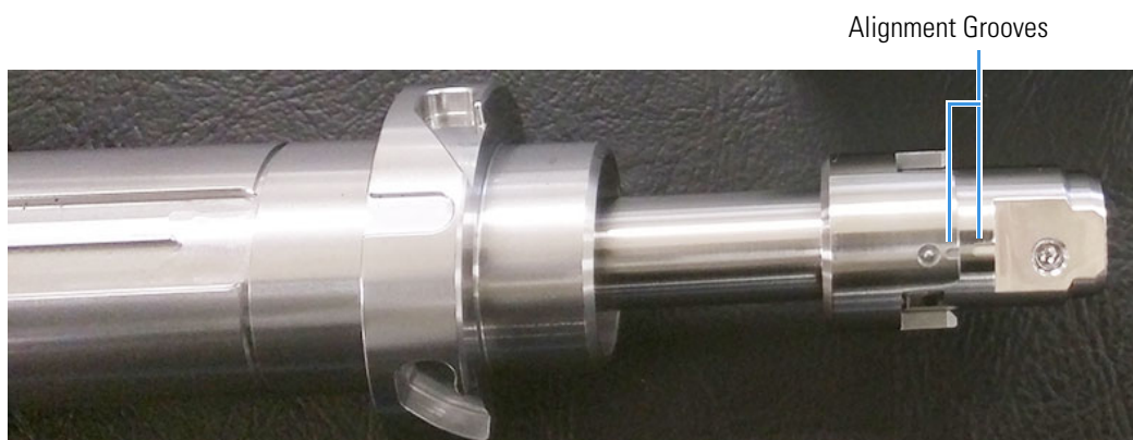
Figure 22. Attaching the V-lock Source Plug to the Source Exchange Tool
