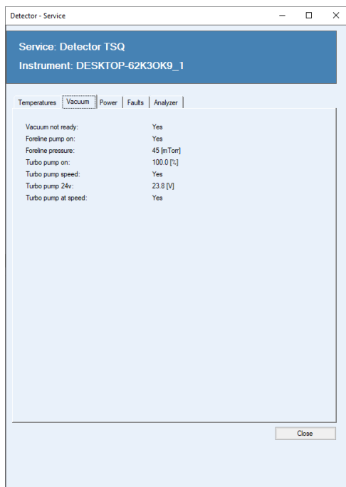
Figure 4. Checking the Vacuum in Chromeleon Software
