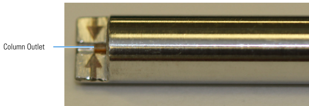
Figure 32. Lining Up the Column in the Column Measuring Tool
