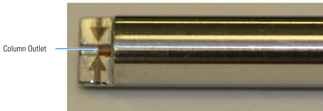
Figure 10. Lining Up the Column in the Column Measuring Tool
