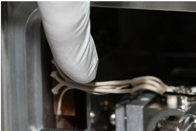
Figure 251. Securing the Source Interface Board Wires
