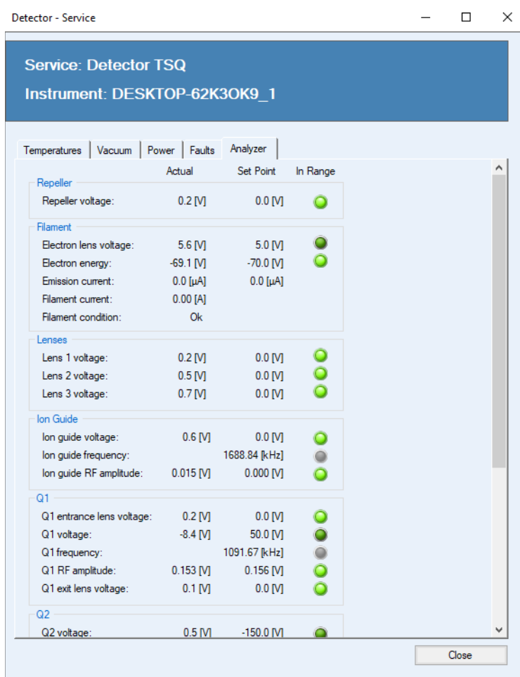
Figure 5. Checking the Status of the TSQ 9610 system in Chromeleon Software
