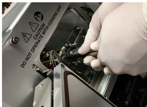
Figure 478. Removing the ExtractaBrite Ion Source
