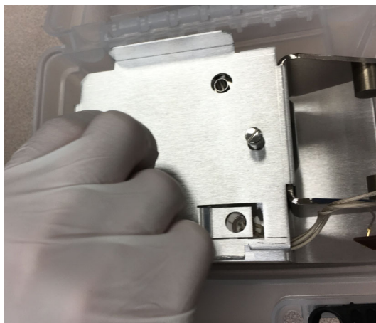
Figure 482. Storing Extra Source Parts in the AEI Source Case
