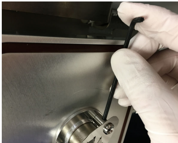
Figure 477. Tightening the Magnets
