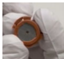
Figure 73. Inserting the Filament Shield into the Filament Insulator
