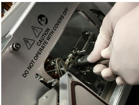
Figure 250. Inserting the Ion Source Cartridge into the Instrument
