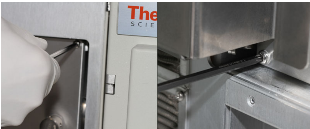
Figure 244. Removing the Manifold Door Screws
