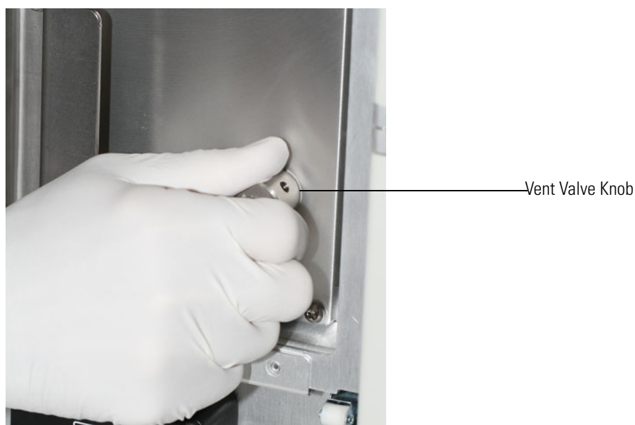
Figure 243. Venting the TSQ 9610 Mass Spectrometer
