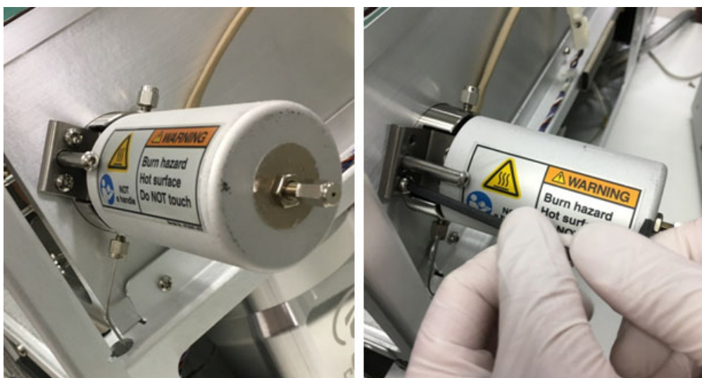
Figure 123. Removing the Transfer Line Screws
