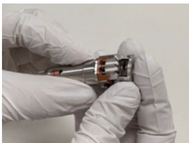
Figure 77. Placing the Cap onto the Filament
