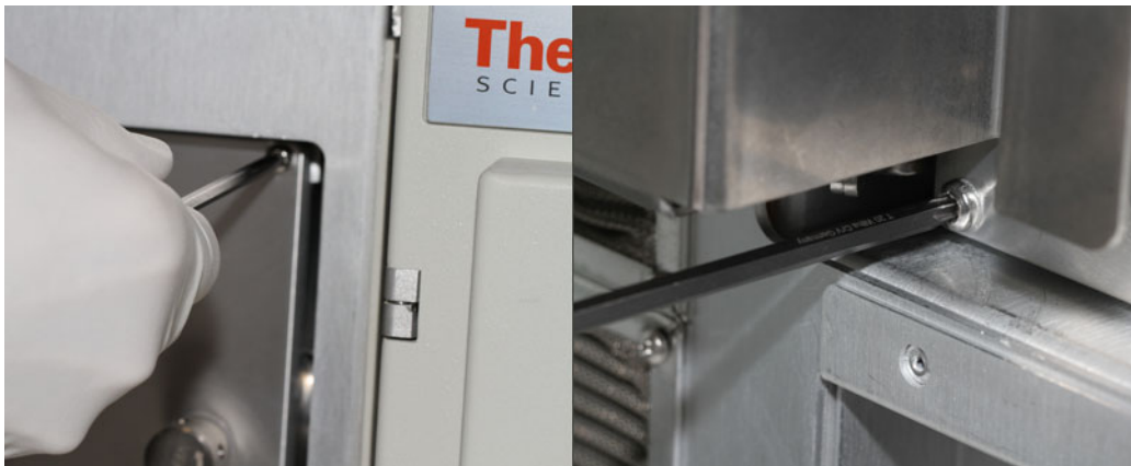
Figure 253. Removing the Manifold Door Screws
