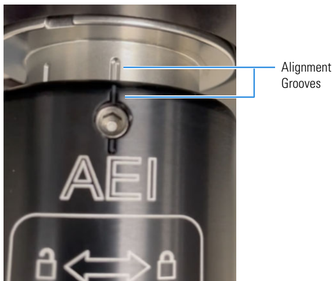
Figure 84. Checking the Alignment on the AEI Source Exchange Tool Before Inserting the NVAEI Ion Source
