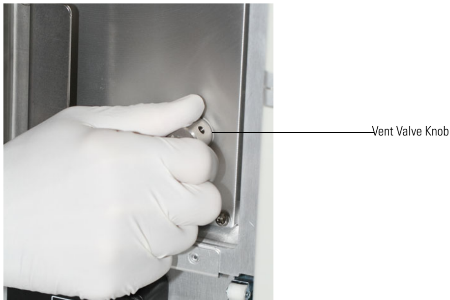
Figure 252. Venting the TSQ 9610 Mass Spectrometer
