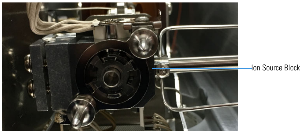
Figure 245. Locating the Ion Source Block
