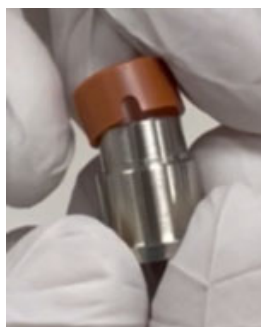
Figure 71. Attaching the Ion Volume Insulator to the AEI Ion Volume
