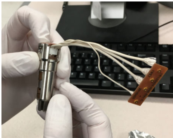
Figure 257. Adding the Filament to the Advanced EI Ion Source Cartridge
