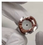
Figure 74. Inserting the Shield and Insulator Assembly into the Ion Cartridge Sleeve
