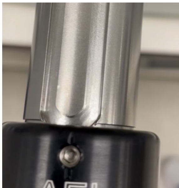
Figure 42. Pulling the AEI Tool to the End of the Track
