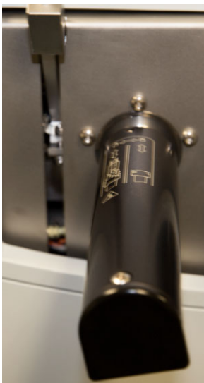
Figure 24. V-lock Source Plug Inserted Correctly
