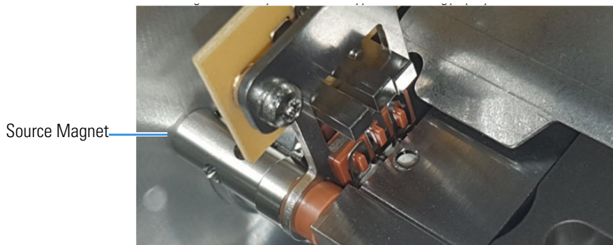
Figure 136. Positioning the Source Magnet Correctly
