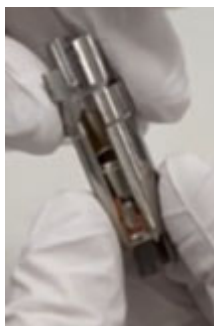
Figure 70. Inserting Lens 2 into the Ion Cartridge Sleeve
