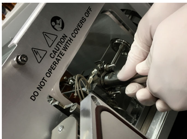
Figure 247. Twisting the Small Source Removal Tool
