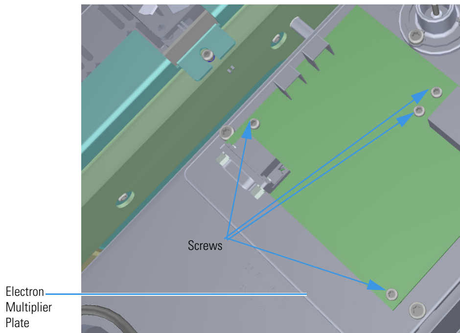
Figure 327. Removing the Electrometer Board
