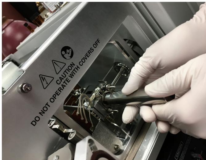
Figure 246. Inserting the Small Source Removal Tool
