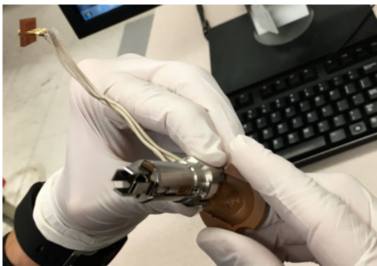
Figure 258. Removing the Ion Source Cartridge
